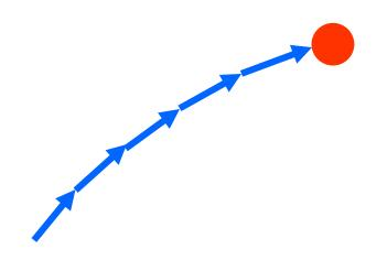
$t = t_5$  a = [0, -9.81, 0]  $v_5 = [10, 5.0950, 0]$  $p_5 = [5, 4.0190, 0]$
