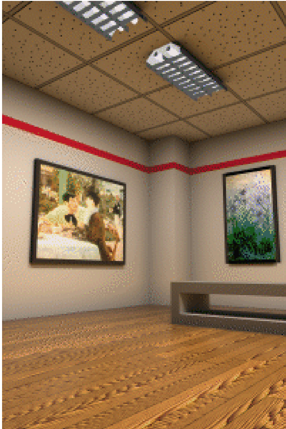
Figure 3.12: An imposter of rectangular luminaire for lighting computation.
