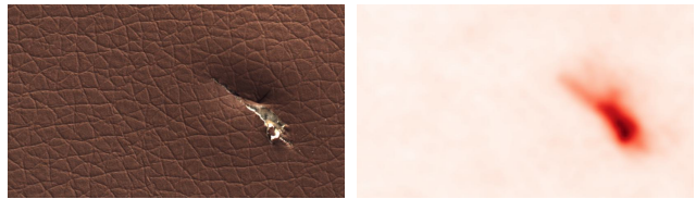
Figure 1. Anomaly localization example. Left : input texture; right : predicted anomaly map.
