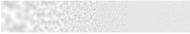
Figure 2: From left to right at the height specified: Perlin noise texture tests with a 1 mm height with level 1 (4x4 grid), level 2 (8x8 grid), level 3 (16x16 grid), level 4 (32x32 grid), level 5 (64x64 grid), and level 6 (128x128 grid)
