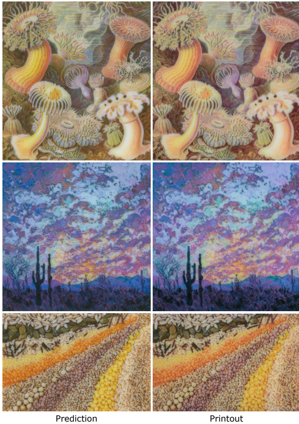
Fig. 15. Predictions of our printouts’ appearance using the measured data from Table 2. The slight blurriness of the printouts’ images is due to the band-limitedness of our optical capture system, plus any residual surface roughness which our surface treatment (Sec. 8) cannot eliminate entirely.
