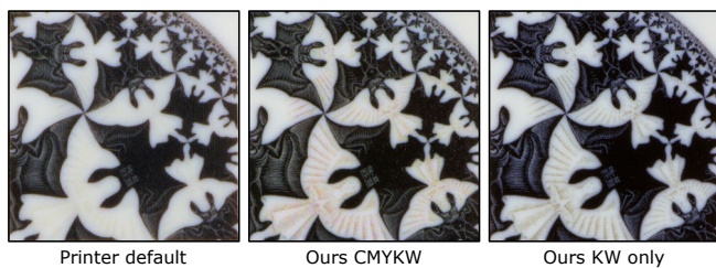
Fig. 20. Comparison of our full CMYKW result and the KW (black and white) only, to the default printer output.
