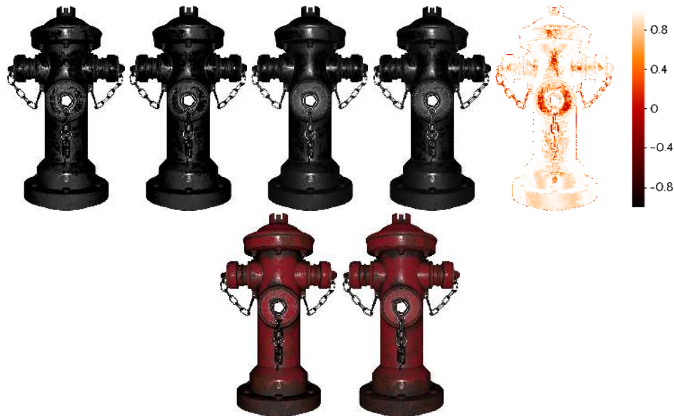
Figure 18. SVR chained remapping from Ward (Blender) to GGX (Cycles) via two intermediate BRDF models. Blender internal-Ward, Mitsuba-Ward, Mitsuba-GGX, Blender Cycles-GGX, SSIM error (left to right); Blender internal-Ward, Blender Cycles-GGX (bottom with diffuse term).
