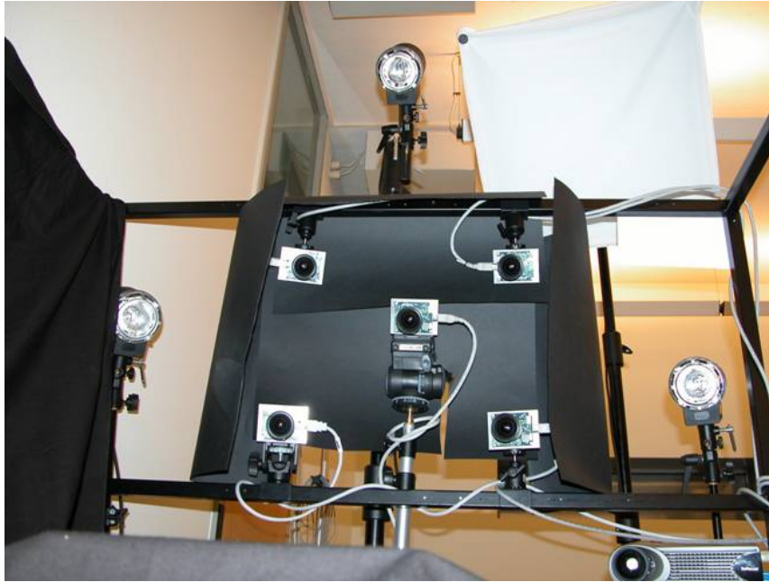
Figure 5.5: 3D reconstruction testbed. We evaluated photometric and active stereo techniques using three light sources, five cameras, and a structured light projector.
