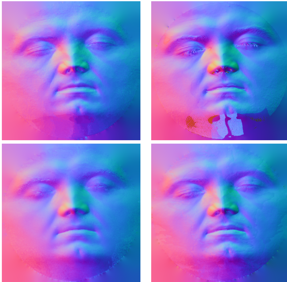
Figure 7.11: Results of the normal estimation step. From left to right, top row: normals from Specular Direction, Helmholtz Stereopsis. Bottom row: photometric stereo with highlight removal, standard photometric stereo.
