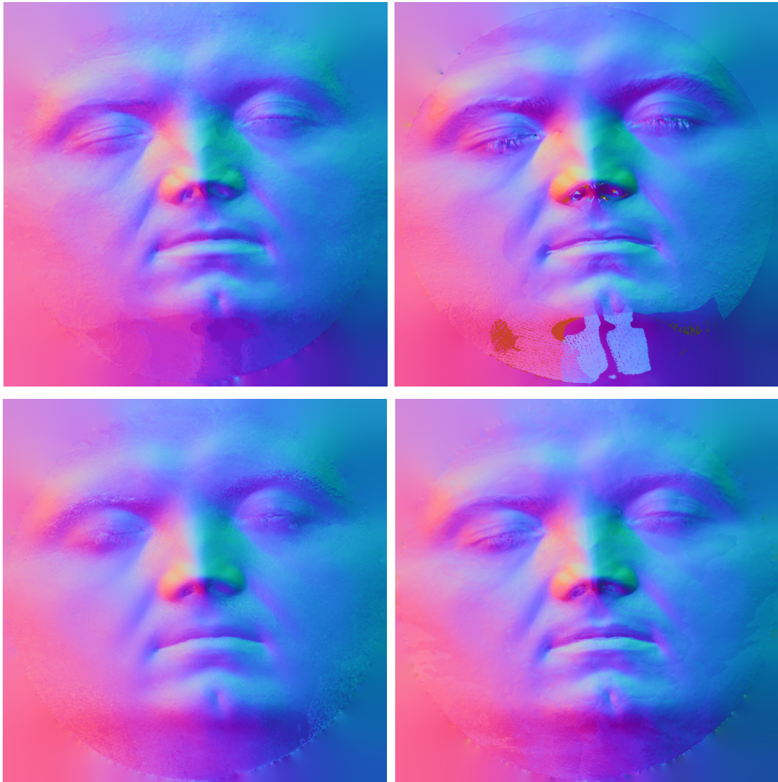
Figure 7.11, page 114: Results of the normal estimation step. From left to right, top row: normals from Specular Direction, Helmholtz Stereopsis. Bottom row: photometric stereo with highlight removal, standard photometric stereo.
