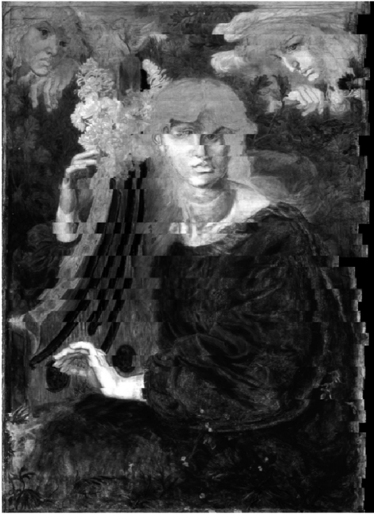
Fig. 19. The SWIR image strips with dropped frames fill left-justified.
