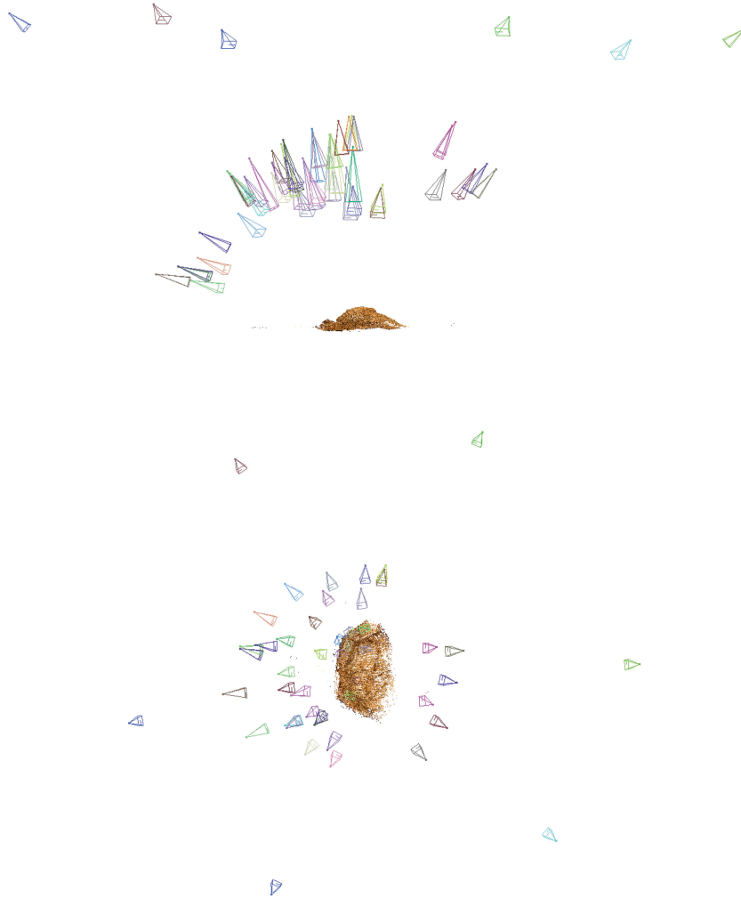
Fig. 6 Screenshot of a visualization of the camera positions used to image a single folio side, indicating the range of movement required around the folio to gain enough coverage of the surface to build a robust model
