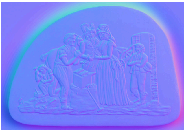
(b) Normal map acquired from RTI acquisition of a sprig mould
