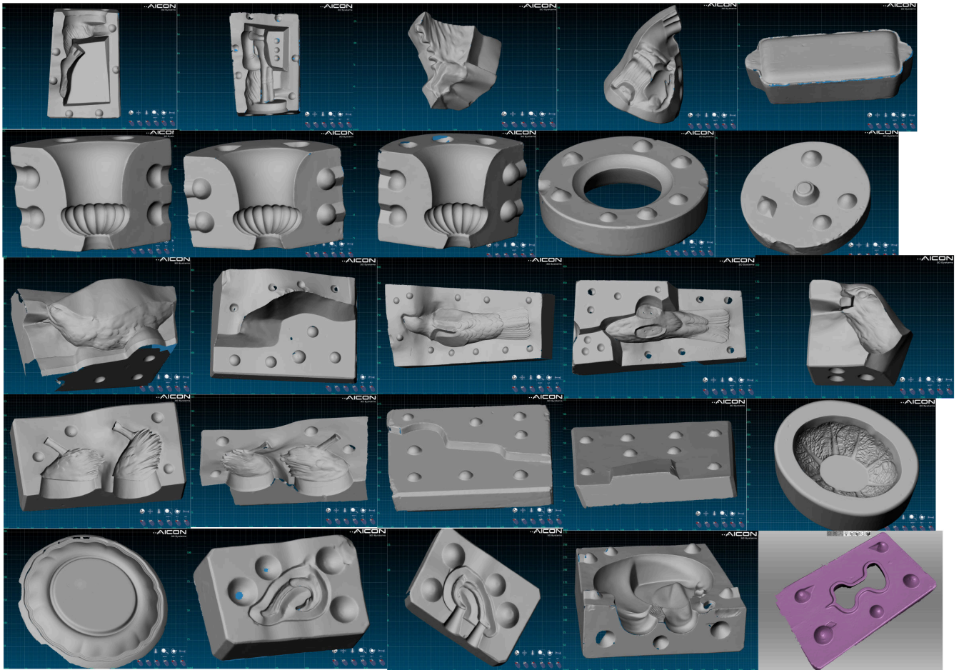
Figure 10: 3D models of scanned moulds.
