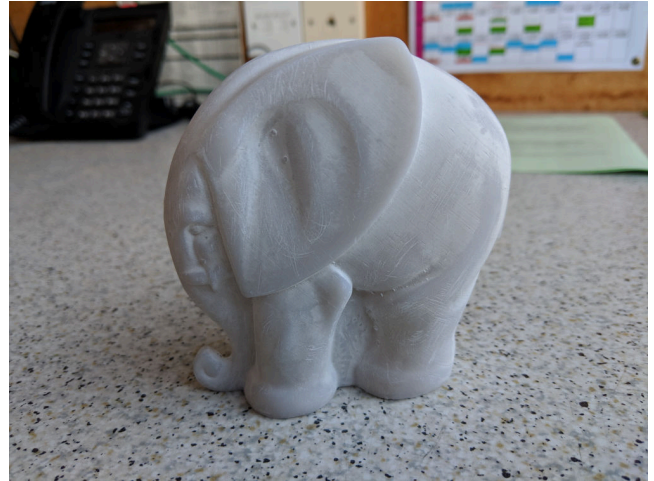
Figure 13: 3D print of African elephant shape after post-processing in IPA (isopropyl alcohol), removed supports and sanded.
