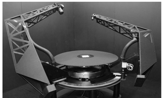
Figure 13: Our custom four-axis gonioreflectometer uses white-LED illumination and a Canon 5DSR 50-megapixel camera to flexibly sample high-dynamic range BTFs at 75 \mu m texel resolution (downsampled from up to 37 \mu m pixels for orthographic views).
