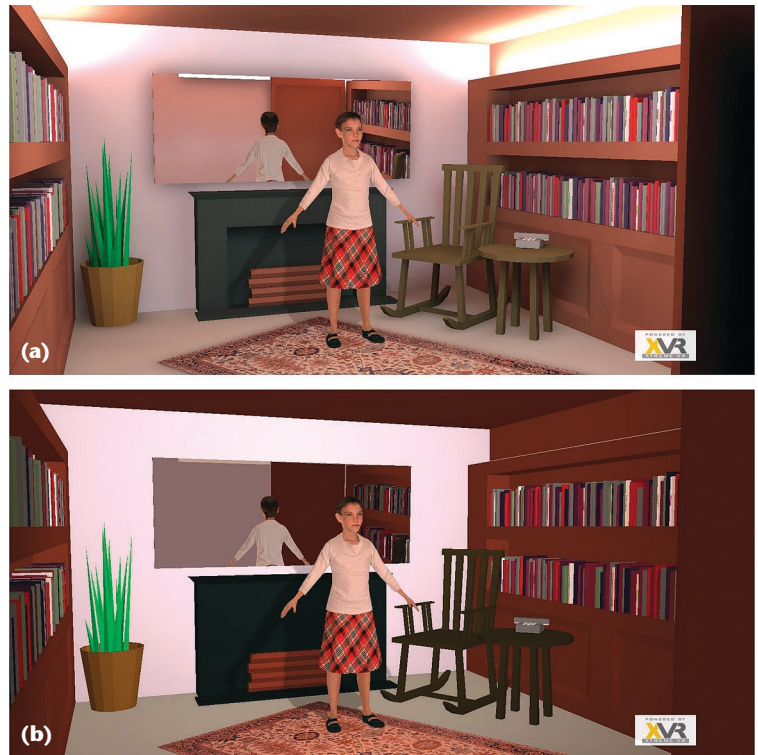
Figure 1. Integrating dynamic elements into a static scene: (a) a virtual character in a globally lit scene showing color bleeding, caustics, and soft shadows, as well as specular reflection; and (b) an OpenGL rendering. Note the realistic appearance due to global illumination effects, in contrast to standard OpenGL rendering, which is commonplace in VR research.
