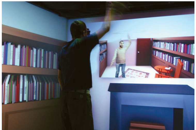
Figure 3. A participant in a CAVE (Cave Automatic Virtual Environment) virtual library application. His virtual body is invisible within the scene but does reflect in the virtual mirror. This illustrates full global illumination with support for tracked dynamic avatars; note the correspondence of the virtual character's pose with the tracked subject.
