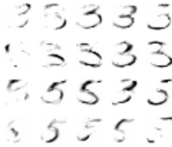
Figure 8. Features that were obtained after learning from a database of 400 handwritten ‘threes’ and ‘fives’. Each of the 4 rows represents an independent set which consists of 4 features and an ‘origin’ feature (most right in each row).
