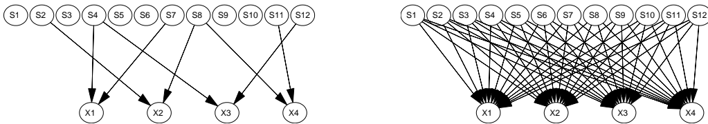
Figure 3. a) GVQ networks with n = 12 features and d = 4 visible units. a) Each visible unit X_i is connected with only two binary parent units ( k = 2 ). b) Fully connected network ( k = n ).
