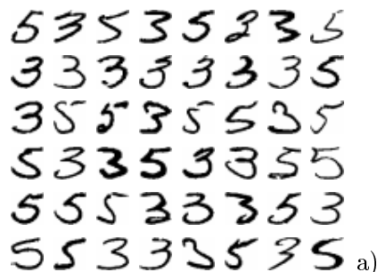
Figure 7. A random sample of 48 handwritten ‘threes’ and ‘fives’ from the CEDAR CDROM. Each image consists of 20 \times 20 bits.
