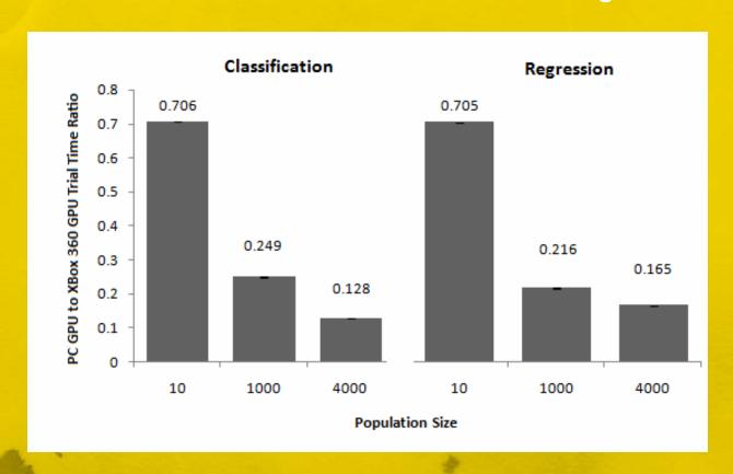
PC GPU to Xbox 360 GPU mean trial time ratios with standard error, based on 10 trials of 50 generations. Ratios of greater than 1 show the Xbox 360 GPU use is faster, less than 1 that the PC GPU is faster.
