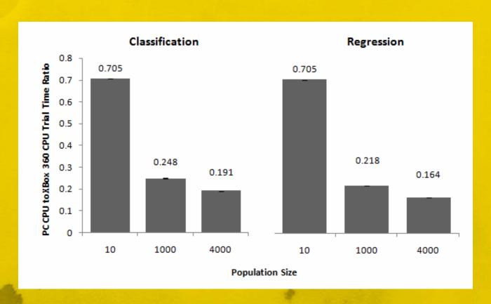
PC CPU to Xbox 360 CPU mean trial time ratios with standard error, based on 10 trials of 50 generations. Ratios of greater than 1 show the Xbox 360 CPU use is faster, less than 1 that the PC CPU is faster.
