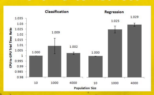
CPU to GPU mean trial time ratios on Xbox 360 with standard error, based on 10 trials of 50 generations. Ratios of greater than 1 show GPU use is faster, less than 1 that CPU is faster.
