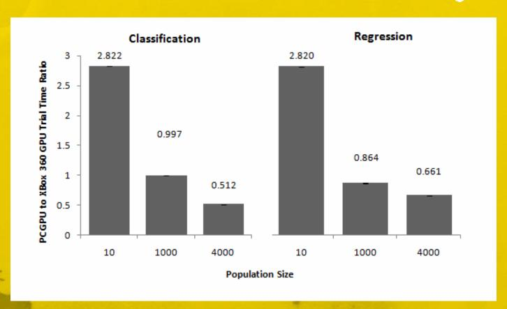
PC GPU to Xbox 360 GPU mean trial time ratios with standard error, normalized to current generation of GPUs, based on 10 trials of 50 generations. Ratios of greater than 1 show the Xbox 360 GPU use is faster, less than 1 that the PC GPU is faster.
