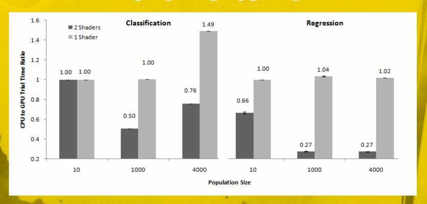
CPU to GPU (both 1 and 2 shaders) mean trial time ratios on PC with standard error, based on 10 trials of 50 generations for classification (left) and regression (right) benchmarks. Ratios of greater than 1 show GPU use is faster, less than 1 that CPU is faster.
