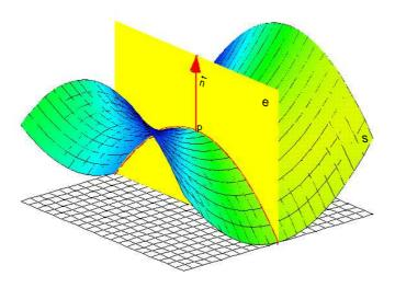
Figure 3.2 A normal plane e with normal vector n intersects saddle surface S, given by function  $f(x,y) = x^2 - y^2$ , at p = (0,0,0).
