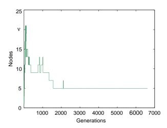
Figure 3.5 Progression of the genotypic size of the best-in-generation genotypes during dowel reconstruction. Genotypic size measured in number  $\nu$  of CSG tree nodes.
