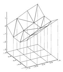
**Figure 3.1**Gridded triangulation of a curved surface. Dotted lines represent normal vectors from uniform grid cross points to corresponding triangle corner points.
