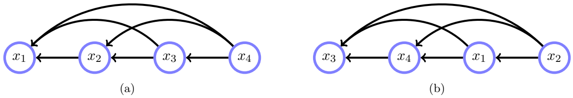
Figure 3.2: Two BNs for a 4 variable distribution. Both graphs (a) and (b) represent the same distribution p(x_1, x_2, x_3, x_4) . Strictly speaking they represent the same (lack of) independence assumptions – the graphs say nothing about the content of the CPTs. The extension of this ‘cascade’ to many variables is clear and always results in a Directed Acyclic Graph.
