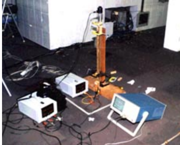
Figure 2-4. Device constructed for measuring system lag.
