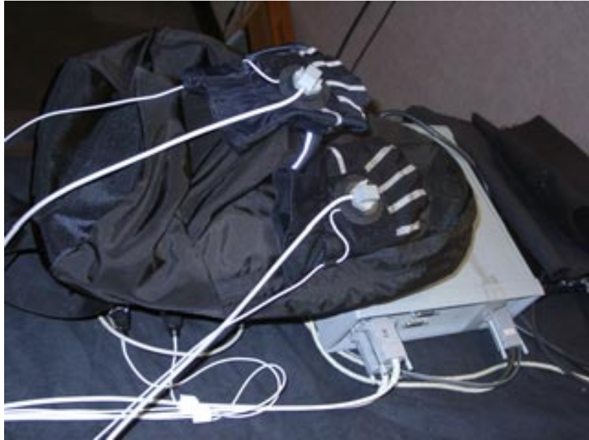
Figure 2-2. Polhemus FastTrak magnetic tracker and equipment.
