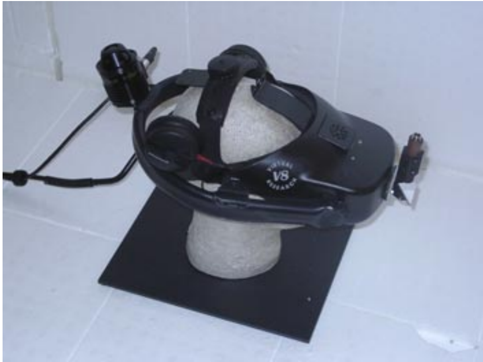
Figure 2-3. V8 Head-Mounted Display with HiBall
